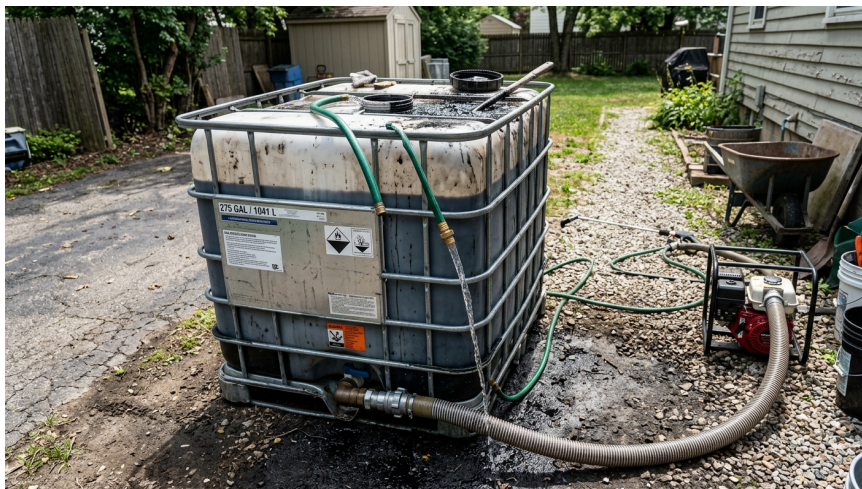
IBC tote for mixing HS concentrate with water
