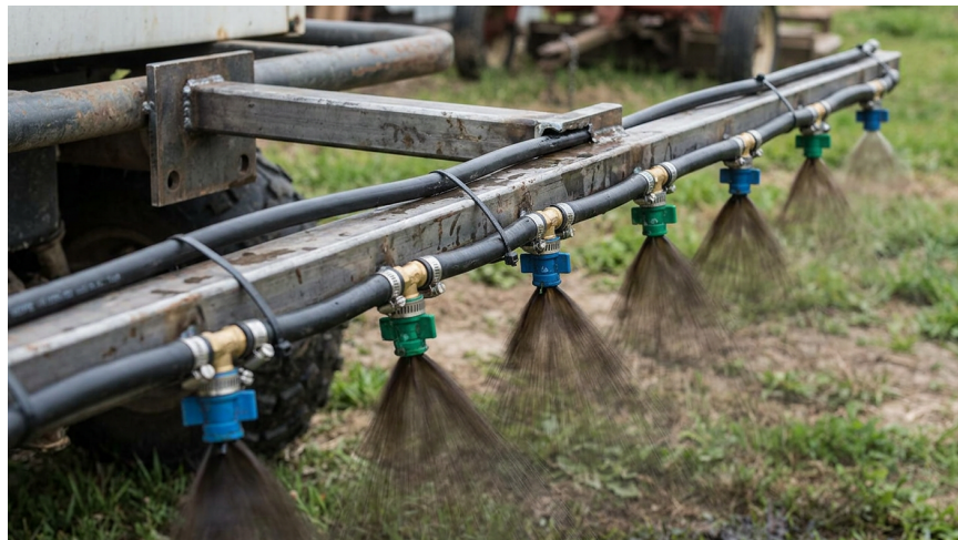
Custom boom with fan jet nozzles mounted every 6–12 inches
